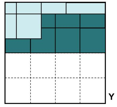
One long pipeline (all cores of a node) advances through the lattice, each update is shifted by (-1,-1,-1)
