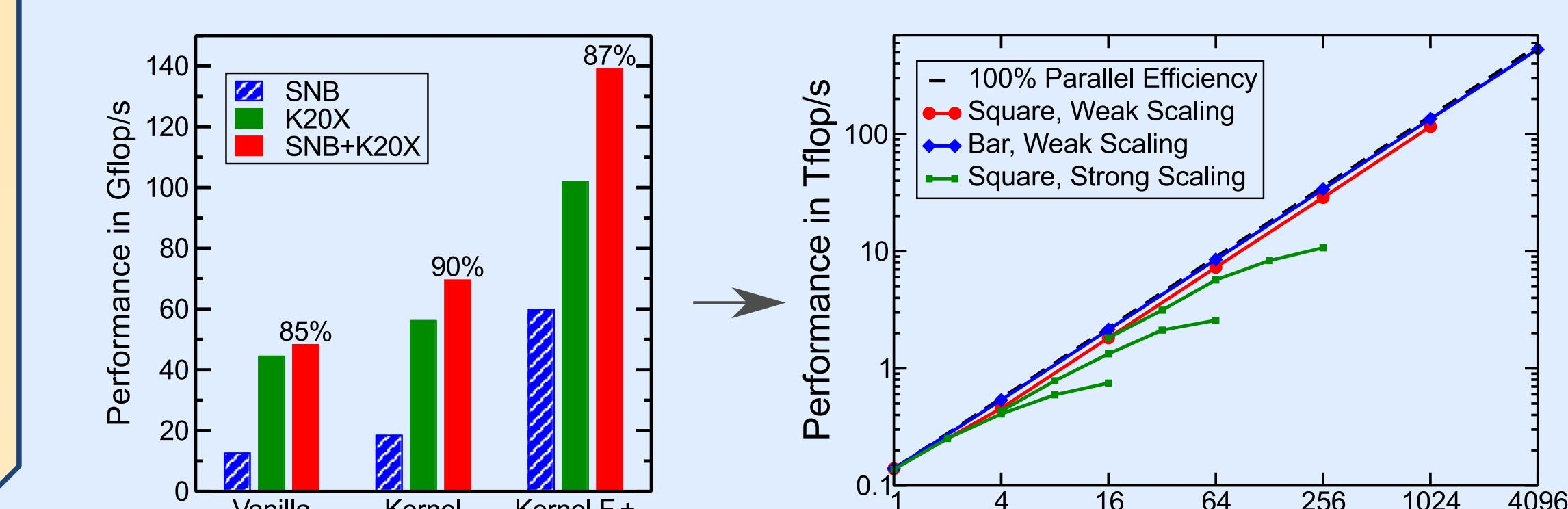
Node-level KPM performance on a single node of Piz Daint (1x Intel Xeon E5-2670, 1x Nvidia Tesla K20X).
