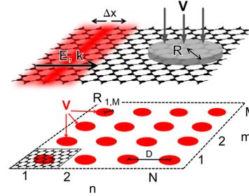
**Schematic representation of the scattering geometry.** Upper panel: An electron wave packet of energy  $E$ , momentum  $k$  and width  $\Delta x$  propagates in a broad graphene sheet. It impinges on a circular, electrostatically defined dot with radius  $R$  and applied potential  $V$ . Lower panel: Graphene quantum dots arranged in a square superlattice with lattice constant  $D$ .
