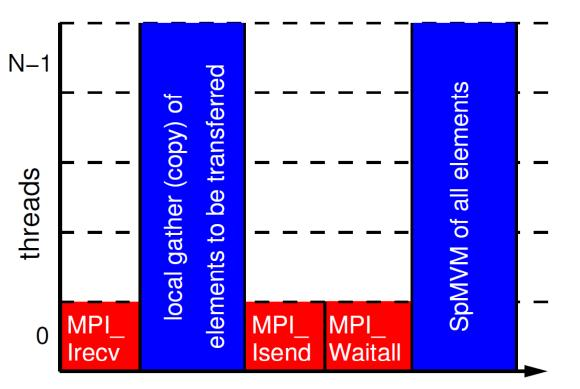
Benefit of threaded MPI process only due to message aggregation and (probably) better load balancing
