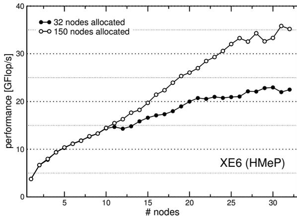
Figure 7: Scaling behavior of HMeP on the Cray XE6 on up to 32 nodes with different numbers of nodes allocated on the 176-node machine.
