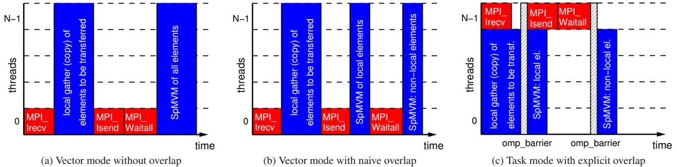
Figure 5: Schematic timeline view of the implemented hybrid kernel versions. From left to right: no communication/calculation overlap, naive overlap using nonblocking MPI, and explicit overlap by a dedicated communication thread
