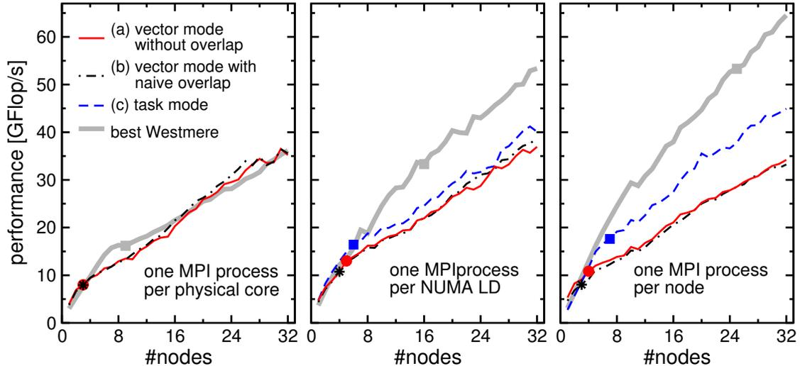
Figure 6: Strong scaling performance data for spMVM with the HMeP matrix on the Cray XE6 for different pure MPI and hybrid variants (kernel version (a) – (c)) as in Fig. 5). Symbols on each data set indicate the 50% parallel efficiency point with respect to the best single-node version. The best variant on the Westmere cluster system (task mode in all cases) is shown for reference (see text for details).
