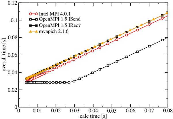
Figure 1: Results for the asynchronous nonblocking MPI benchmark for several MPI implementations on a Westmere-based cluster with QDR InfiniBand interconnect (internode communication). Overlap does generally not work for intranode communication. Unless indicated otherwise, results for nonblocking send and receive are almost identical.
