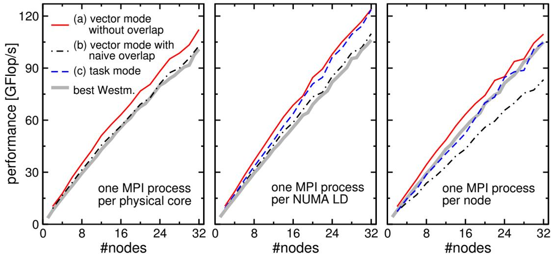
Figure 8: Strong scaling performance data for spMVM with the sAMG matrix (same variants as in Fig. 6). Parallel efficiency is above 50% for all versions up to 32 nodes. The Westmere cluster performed best in vector mode without overlap for all cases, just like the Cray XE6.
