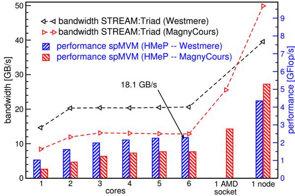
Figure 4: Node-level performance for the Westmere and Cray XE6 test systems. Effective STREAM triads bandwidth<sup>1</sup>, and performance for sparse MVM using the HMeP matrix (bars) is shown.
