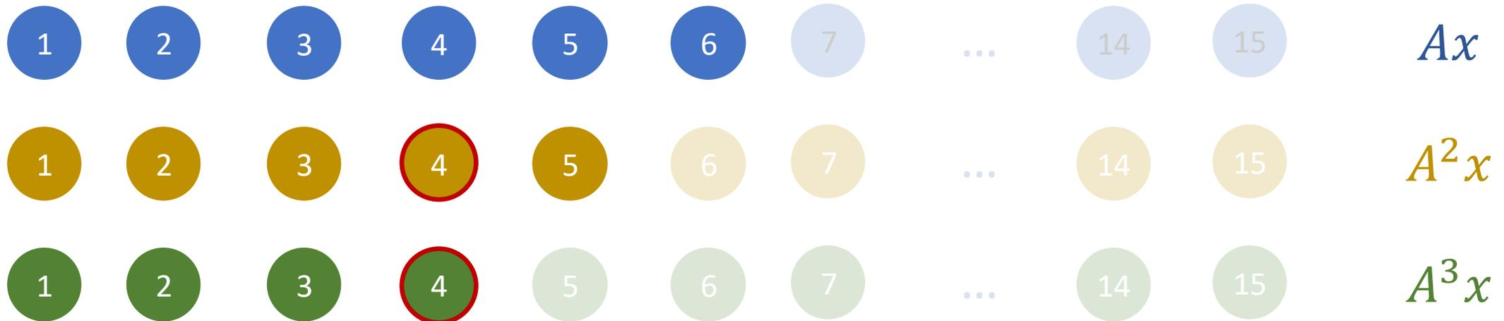
A is loaded only once if  $(p + 1) \times N_{nz}(L) \times 12 \text{ bytes} < C$
