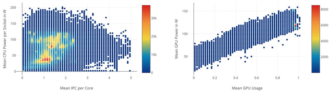
Figure 4.7: Performance footprint visualization as scatter plots (*Performance Maps*) for a period of one year on TU Dresden's Taurus system. The chart on the left compares *IPC* and *CPU Power* and shows a hot spot for *IPC=1* and *CPU Power=40* watts. The chart on the right compares *GPU Usage* and *GPU Power* and illustrates that as the GPU usage increases, the power increases proportionally.
